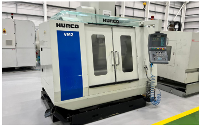
29480 HURCO VM2 Vertical Machining Centre with Nikken CNC202YA 4th Axis Attachment. Year 2006.
