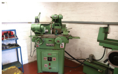
29904 MYFORD MG12 Cylindrical Grinder with Internal Grinding Attachment
