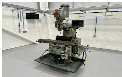
29812 BRIDGEPORT Series 1 2HP Variable Speed Turret Mill with DRO
