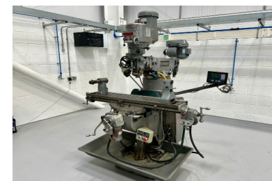
29815 BRIDGEPORT Series 1 2HP Variable Speed Turret Mill with Slotting Attachment and DRO
