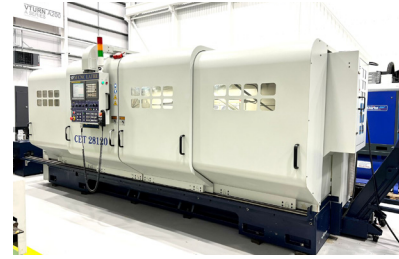
29553 SFM Model CET28120 CNC Flat Bed Lathe with Fanuc 0i-TD Control. Year 2014
