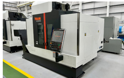
29788 MAZAK VCN 530C Vertical Machining Centre with Smooth Control. 18k spindle. c/w Ultraspindle attachment. Year 2022
