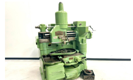
29789 MAXICUT 3A Gear Shaping Machine with Spur & Helical Guides, 6" Riser Block & Change Gears
