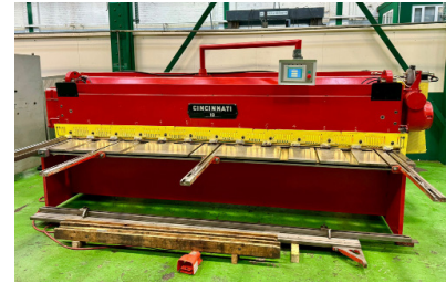
28339 CINCINNATI 1012 Auto Shear. Capacity 12' x 10swg. Recently fully rebuilt with Siemens Simatic Touch Screen NC Backgauge
