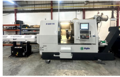
29785 BIGLIA Model B620 YS CNC Lathe with C Axes, Y Axis and Sub Spindle. Fanuc 0i-TF Control. Year 2021
