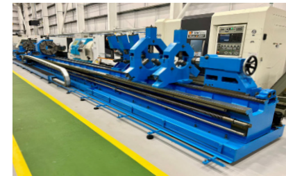
28729 BINNS & BERRY Trident L850 Straight Bed Centre Lathe x 12,000mm Between Centres. Rebuilt 2008
