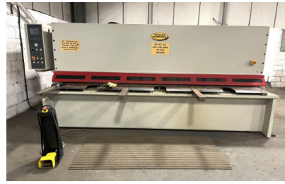
29948 MORGAN RUSHWORTH BHG3 3100 x 10 Hydraulic Guillotine with Cybelec CybTouch 8 NC Controller. Year 2013
