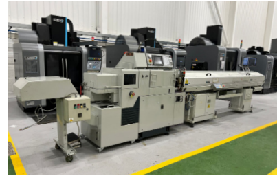
29296 CITIZEN B12 Sliding Head CNC Lathe with IMECA Mini Boss 325CNC Barfeed. Year 1997
