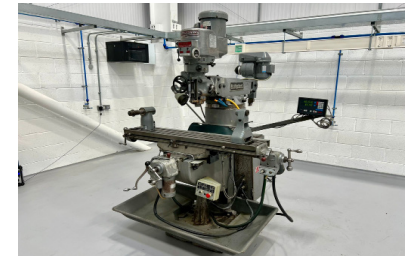
29815 BRIDGEPORT Series 1 2HP Variable Speed Turret Mill with Slotting Attachment and DRO
