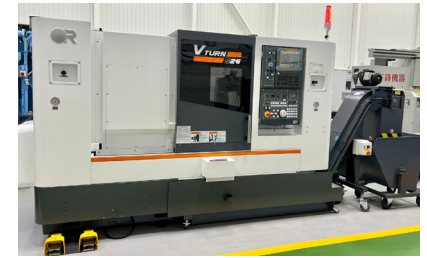
10045 NEW VICTOR S26/60 LSB Horizontal Turning Lathe with Fanuc 0i-TF Plus Control
