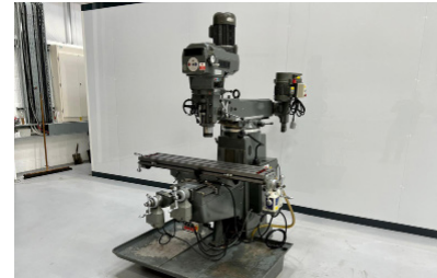
29370 AJAX Model AJT1 Turret Milling Machine
