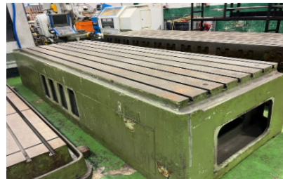
29926 CAST IRON Boxtable 3810mm x 1092mm x 812mm. Weight 6.5 ton CHOICE OF 2
