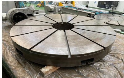
29562 T Slotted Heavy Duty Cast Iron Circular Sub Table 2540mm dia. x 310mm thick
