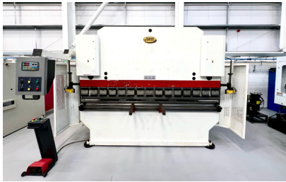
29947 MORGAN RUSHWORTH PBNC 3100-160 Hydraulic Downstroking Pressbrake. Year 2013
