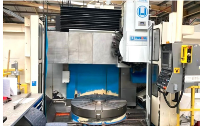
29945 TOS Hulin SKIQ16 CNC Vertical Borer with Fanuc 16T Control. Year 1999
