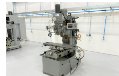
29120 SEMCO LC-50RS Milling Machine with Heidenhain DRO
