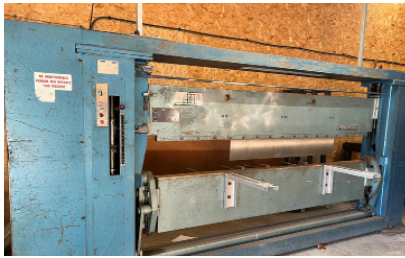
29954 KEETONA 100" x 0.125" Hydroform Powered Folder. Year 1981
