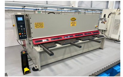
29948 MORGAN RUSHWORTH BHG3 3100 x 10mm Hydraulic Guillotine with Cybele CybTouch 8 NC Controller. Year 2013
