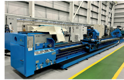
28729 BINNS & BERRY Trident L850 Straight Bed Centre Lathe x 12,000mm Between Centres. Rebuilt 2008
