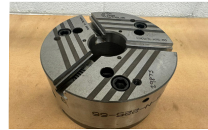
29875 USED SMW AUTOBLOK KNCS-N-225-66 3 Jaw Powered Chuck. 9" Diameter. Various sizes available
