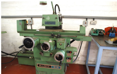
29903 ELLIOTT Model 618 Hydraulic Surface with Magnetic Chuck
