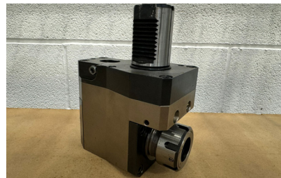
29885 MT SAUTER Revolver DN5480 VDI40 Driven Tool Holder
