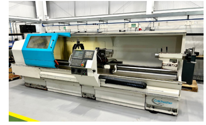
30063 COLCHESTER Multiturn 4000 CNC Gap Bed Lathe with FANUC 0i-TC Control. Year 2005
