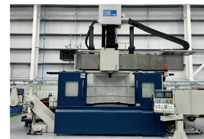
29474 HNK Model VTC14/16 Vertical Turning Centre with Fanuc 18i-TB Control. Year 2011
