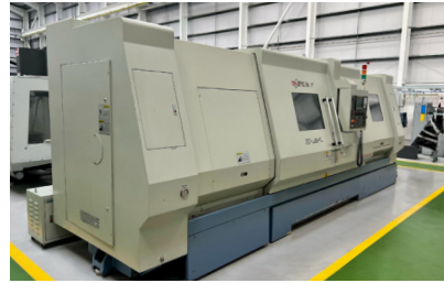
30037 FORCE ONE TC-3523 x 2300mm CNC Slant Bed Lathe with Fanuc Series 0i-TD Control. Year 2012
