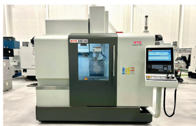
30064 XYZ 800HD Vertical Machining Centre with Siemens 828D Shop Mill Control. Year 2021
