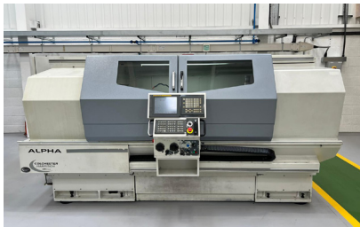
29364 HARRISON Alpha 1460XS CNC Lathe with Fanuc 0i-TD Control. Year 2013
