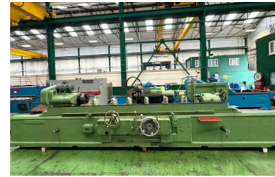
29898 LANDIS LUND HMPB 14/125 Cylindrical Grinder with Angular Table. Complete with Coolant Tank. Filtration. Steadies
