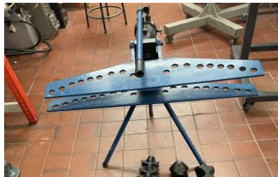
29905 Manual Hand Hydraulic Pipe Bender complete with Formers
