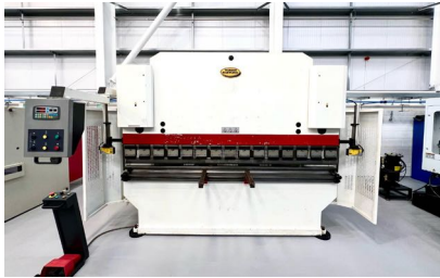
29947 MORGAN RUSHWORTH PBNB 3100-160 Hydraulic Downstroking Pressbrake. Year 2013
