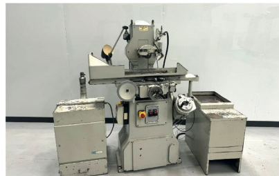
29492 JONES & SHIPMAN 540P Hydraulic Surface Grinder with Magnetic Chuck
