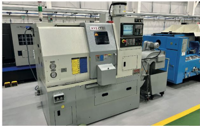
29935 XYZ CT52 CNC Lathe with Siemens Sinumerik 828D Shopturn Control. Year 2015
