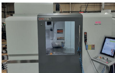
30086 XYZ 1100HD Vertical Machining Centre with Heidenhain Control. Year 2021
