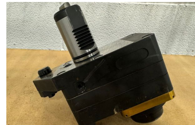
29883 MAZAK Axial Driven Tool Holder. VDI 40
