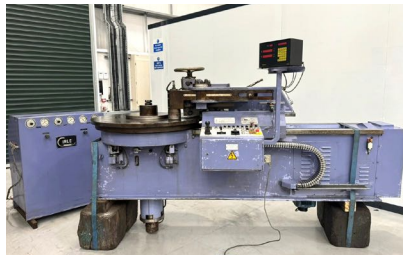
29524 IRLE Model B100 HHG Hydraulic Ring/Section Rolling Machine. Year 1993
