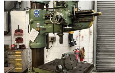
29951 ARCHDALE 3'6" Radial Arm Drilling Machine with Box Table
