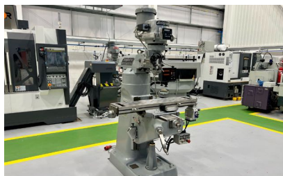
30051 BRIDGEPORT Series 1 2HP Variable Speed Turret Mill with Riser Block & DRO
