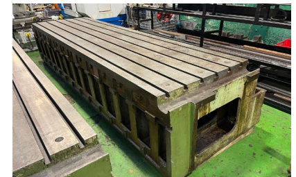
29927 CAST IRON Boxtable 3810mm x 1092mm x 812mm. Weight 6.5 ton
