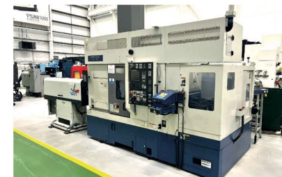
30058 MORI SEIKI SL-153SY 5 Axis CNC Lathe with Collet Chuck, Sub Spindle, Overhead Gantry. MSG - 501 (FANUC) CNC Control Year 2001
