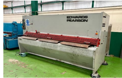
29557 EDWARDS PEARSON Model V13/3000 Hydraulic Guillotine with Cybele DNC60 NC Backgauge
