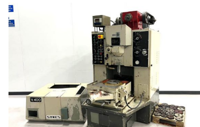
29556 SYKES V400 Gear Shaper with Change Gears
