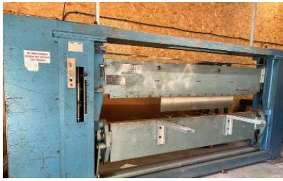
29954 KEETONA 100" x 0.125" Hydroform Powered Folder. Year 1981
