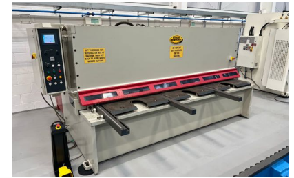
29948 MORGAN RUSHWORTH BHG3 3100 x 10mm Hydraulic Guillotine with Cybelec CybTouch 8 NC Controller. Year 2013
