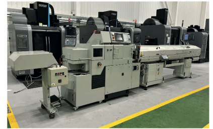
29296 CITIZEN B12 Sliding Head CNC Lathe with IMECA Mini Boss 325CNC Barfeed. Year 1997
