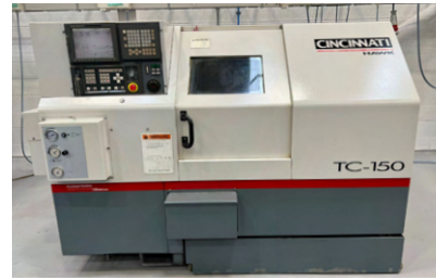
30156 CINCINNATI Hawk TC150 CNC Lathe with Fancu 21i-T Control. Year 2001
