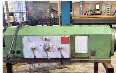
30119 BUTLER Elgammill CS10 Ram Slide Assembly with Vertical Attachment
