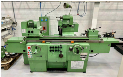
29934 TOS Hostivar BHU 25 x 1000mm Universal Cylindrical Grinder with Internal Attachment
