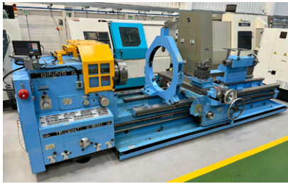
30048 BINNS & BERRY Trident L850 Centre Lathe x 120" Between Centres with Hydraulic Copying and DRO – Rebuilt 2009
