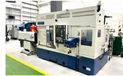
30058 MORI SEIKI SL-153SY 5 Axis CNC Lathe with Collet Chuck, Sub Spindle, Overhead Gantry. MSG - 501 (FANUC) CNC Control. Year 2001
