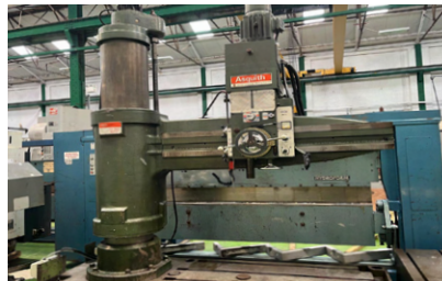
30079 ASQUITH ODI Mk2 16-72" Radial Arm Drilling Machine with Cast Iron Box Table & Safety Brake. Year 1978
