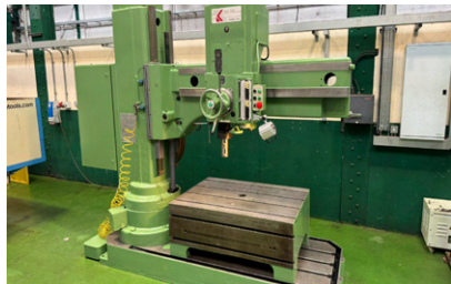
30146 KITCHEN & WALKER KWM 50-1600 Radial Arm Drilling Machine with Cast Iron Box Table. Year 1996
