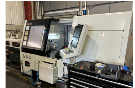
30180 XYZ S565 CNC Lathe with SubSpindle, Live Tooling & Y Axis. Siemens Touchscreen Control. Year 2023
