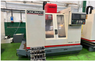
30155 CINCINNATI Dart 500 Vertical Machining Centre with Fancu 21i-M Control. Year 2005
