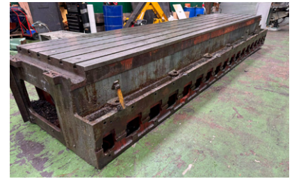
30165 CAST IRON T Slotted Box Table 5350mm x 1090mm x 820mm
