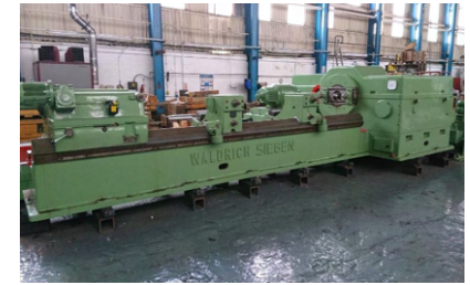
28420 WALDRICH SEIGEN Model WSIIa850 Roll Grinding Machine. Swing 1100mm x 3500mm
