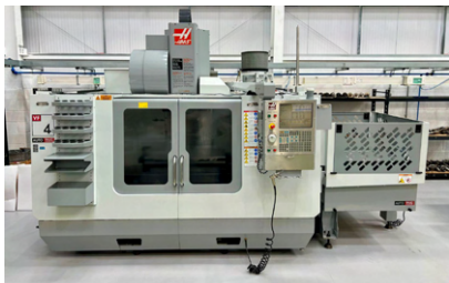
30170 HAAS VF4 APC Vertical Machining Centre with 4th Axis Attachment. HAAS Control. Year 2008
