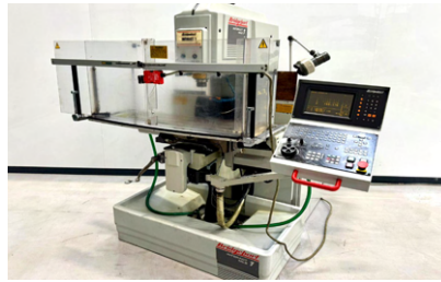
30166 BRIDGEPORT Interact 1 Mk2 CNC Vertical Milling Machine with Heidenhain Control. Year 1996
