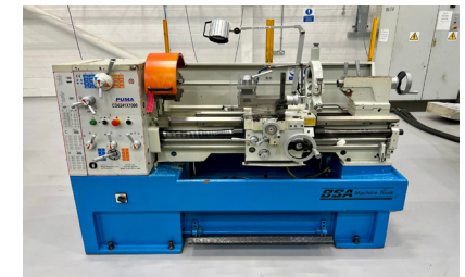
30198 BSA CD6241 x 1010mm Between Centres Gap Bed Centre Lathe with Taper Turning. Ex Training School. 4 Available
