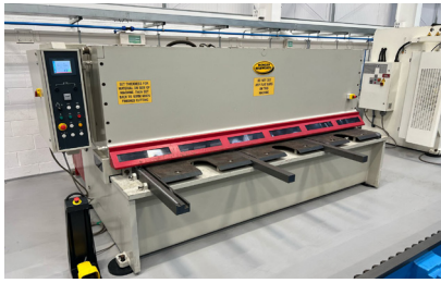
29948 MORGAN RUSHWORTH BHG3 3100 x 10mm Hydraulic Guillotine with Cybelelec CybTouch 8 NC Controller. Year 2013
