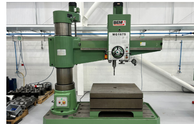
30183 BEMA MG1675 Radial Arm Drilling Machine with Cast Iron Box Table & Safety Brake. Year 2014
