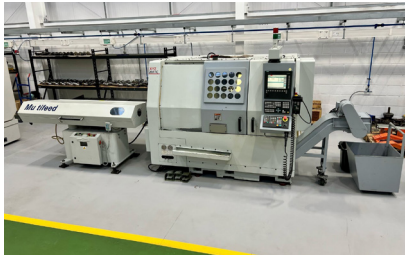
30065 XYZ 200TC CNC Lathe with Siemens 810D CNC Control. Barfeed and Swarf Conveyor
