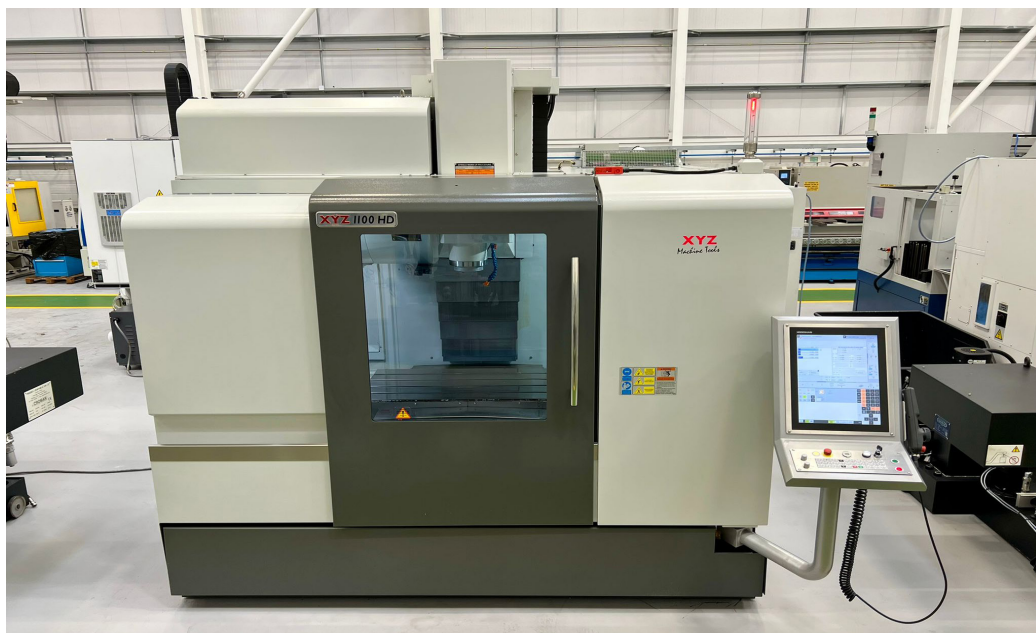
30086 XYZ 1100HD Vertical Machining Centre with Heidenhain Control. Year 2021
