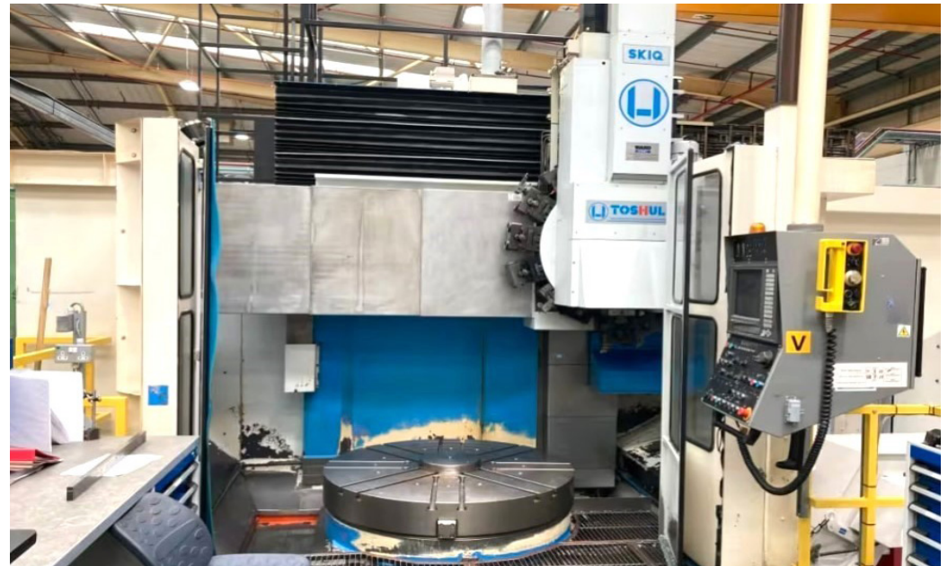
29945 TOS Hulin SKIQ16 CNC Vertical Borer with Fanuc 16T Control. Year 1999
