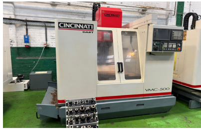
30155 CINCINNATI Dart 500 Vertical Machining Centre with Fanuc 21i-M Control. Year 2005
