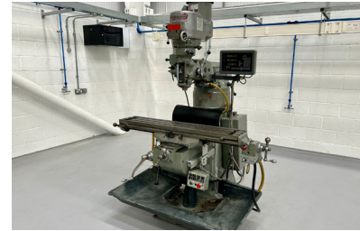
29812 BRIDGEPORT Series 1 2HP Variable Speed Turret Mill with DRO. Year 1976
