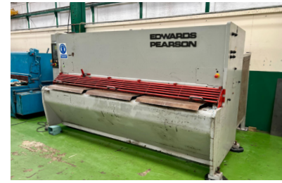
29557 EDWARDS PEARSON Model V13/3000 Hydraulic Guillotine with Cybelelec DNC60 NC Backgauge
