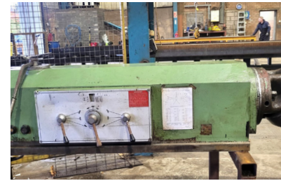
30119 BUTLER Elgamill CS10 Ram Slide Assembly with Vertical Attachment
