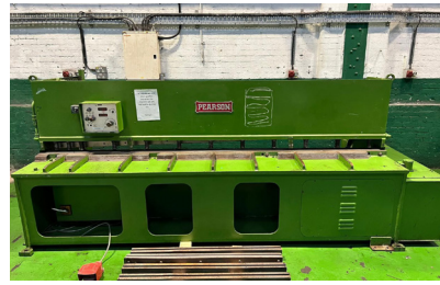
28959 PEARSON 3048mm x 6.5mm Hydraulic Guillotine
