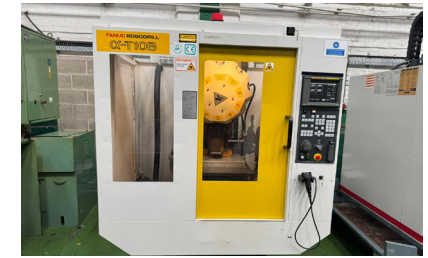
30163 FANUC Robodrill Alpha T10B with Fanuc Control. Year 1995
