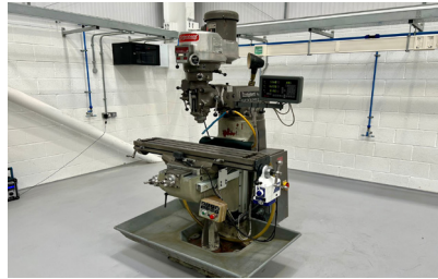
29813 BRIDGEPORT Series 1 2HP Variable Speed Turret Mill with DRO. Year 1979
