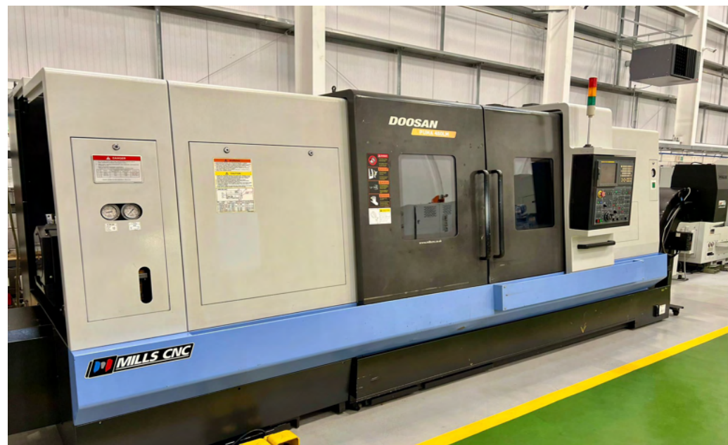
30235 DOOSAN Puma 480LM CNC Lathe with Live Tooling. Fanuc 21i-TB. Swarf Conveyor. Year 2010
