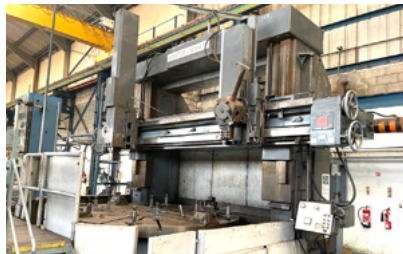
29132 WEBSTER & BENNETT DCM 120" Double Column Vertical Boring Machine with 2 x Newall DP700 Digital Readouts
