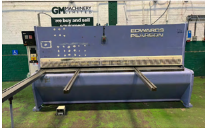
29449 EDWARDS PEARSON Model VE10/3000 Hydraulic Guillotine with Swissax 2000 NC Backgauge. Year 1993
