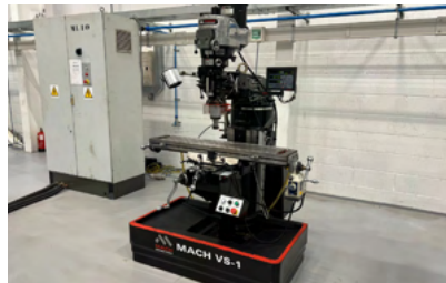
30303 MACH VS-1 Turret Milling Machine with Newall DP700 Digital Readout. Year 2014
