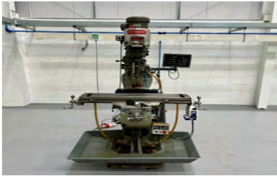
29814 BRIDGEPORT Series 1 2HP Variable Speed Turret Mill with Newall Topaz 2 Axis DRO. Year 1987
