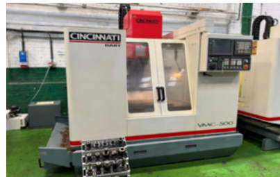
30155 CINCINNATI Dart 500 Vertical Machining Centre with FANUC 21i-M Control. Year 1999
